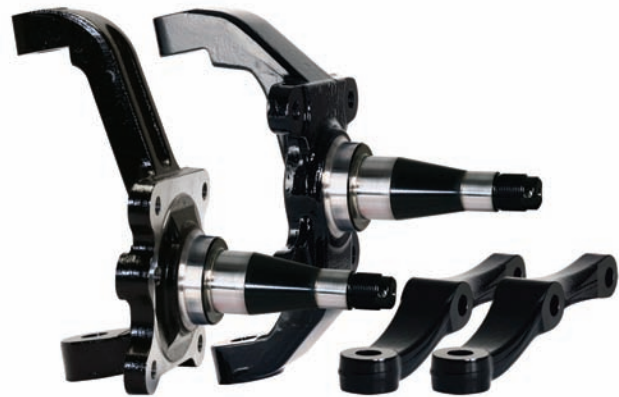
Standard Height Shown Left, 2" Drop Shown Right
